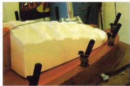
Topper hull assembly showing buoyancy mouldings showing welding braid being fitted. The computer welder is pictured in the background
