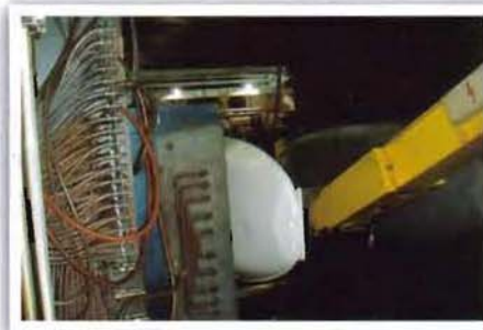
Hull tool showing cooling arrangement and robot arm extracting a moulding
