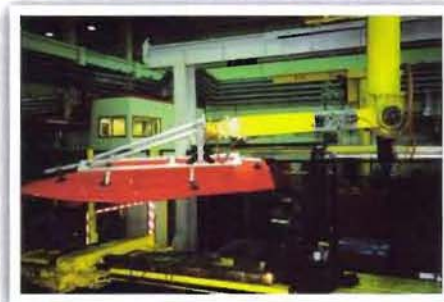
Robot arm removing deck moulding prior to manual trimming
