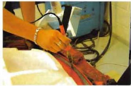
Topper hull assembly showing welding braid being fitted
