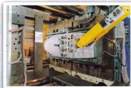
Deck tool separated after removal of moulding
